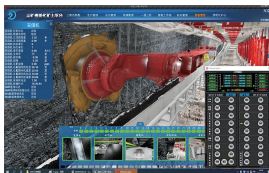
(b) 智能化煤矿综采工作面开采管控应用 (b) Application of intelligent control in intelligent coal mining fully mechanized face
